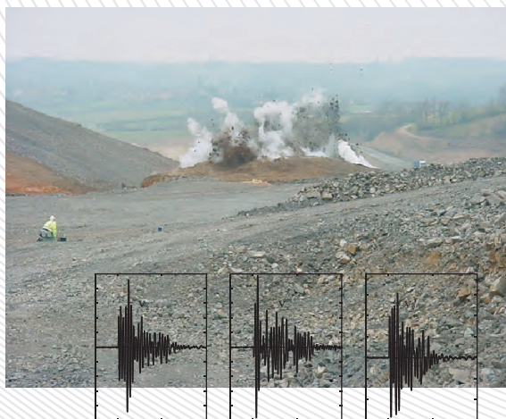
Blast induced vibrations in soils (picture and recorded velocities)
